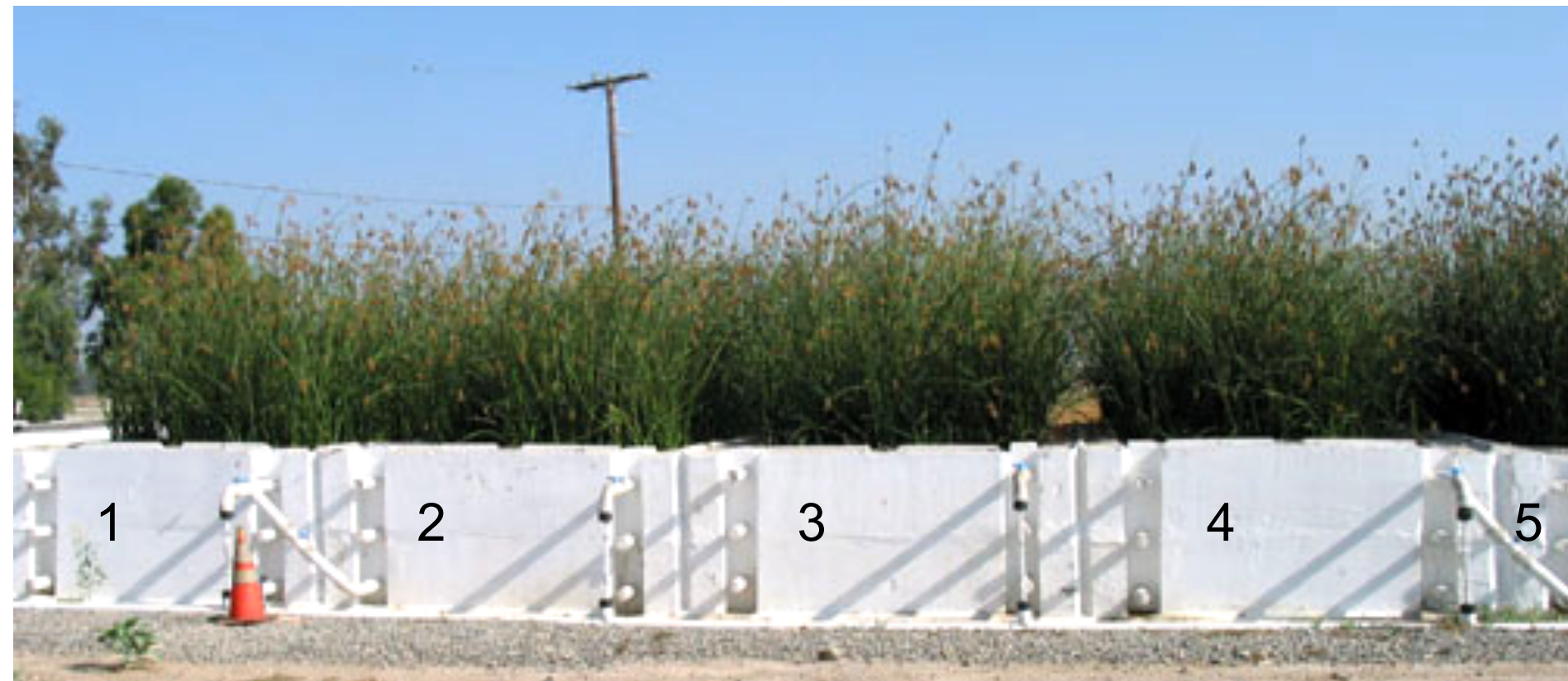
SSF Constructed Wetlands at the OCWD FRL, July 2004. Cells 1-6 received 2, 4, 8, 12, 15 L/minute of Santa Ana River Water.
